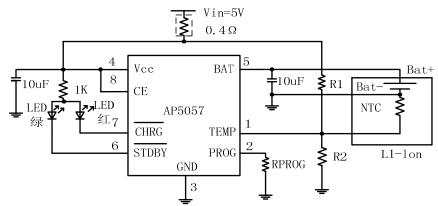
Figure 1. Basic Application Circuit with AP5057
