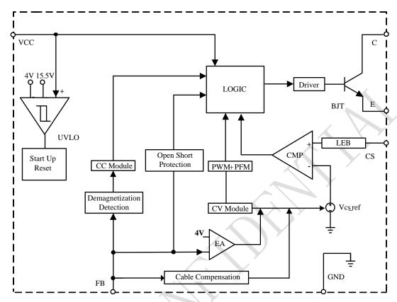
Figure 3: Internal Block Diagram
