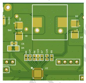
2. Kelvin connection should be used to arranging the current sensing traces, pulling them inward from the resistor pad and leading to the CSP\_VBAT and CSN\_VBAT pins separately, without leading to other places in the route. Similarly, traces on the VBUS side, with a width of 8 mil or 10 mil, should be directly connected to the CSP\_VBUS and CSN\_VBUS pins through the sensing resistors; the 0.1uF capacitor in parallel with the sensing resistor is placed near the sensing resistor.
