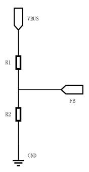
For the settings of output current limit and battery undervoltage threshold, please refer to "10.4.3
