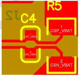
3. General signal traces (not carrying high currents) should have a width of 0.2mm (8mil) or 0.25mm (10mil), and other traces from the chip's HD1, LD1, SW1, HD2, LD2, and SW2 pins to the power components should be at least 0.25mm (10mil) or more in width.
